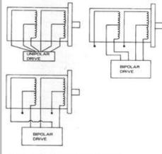
Can be driven from unipolar or bipolar drives.
