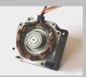
Other motors have only **four leads**: these are not bifilar wound and therefore cannot be used with a unipolar drive. Internally, four wire motors may be
