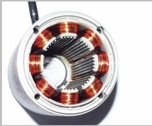
**Full-step** mode in single phase is when the motor is operated with only one phase energised at a time. This requires the least power from the driver power supply, and can be used where the motor is operated at a fixed speed. Dual phase provides increased torque, but uses more power.
