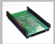
Eurocard circuit boards can slide into internal card guides enabling power devices to be attached to the thick heatsink section of the vertical wall with an M3 screw and half nut.
