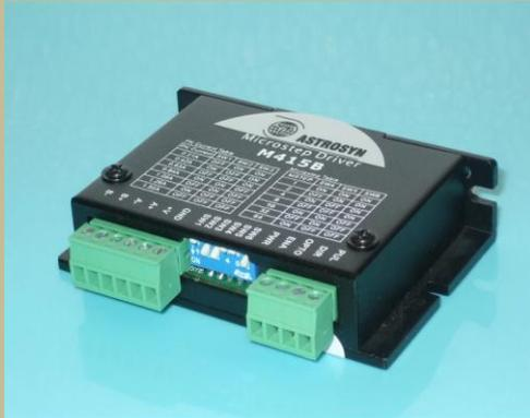
Other firmware functions included in these units include microstep emulation, torque ripple smoothing and command signal smoothing. With microstep emulation, low resolution systems can still provide smooth motion as the drive can modify low resolution step pulses and create fine resolution motion.
