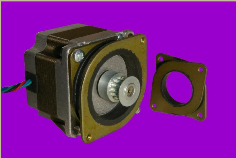
normally consist of a lightweight housing, which is fixed rigidly to the motor shaft, and an inertia ring, which can rotate relative to the housing. The ring and the housing are mechanically isolated by a viscous gel or by an elastomer disc.
